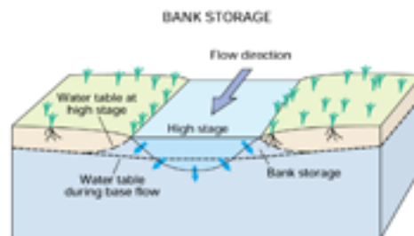
Figure 11. If stream levels rise higher than adjacent ground-water levels, stream water moves into the streambanks as bank storage.
